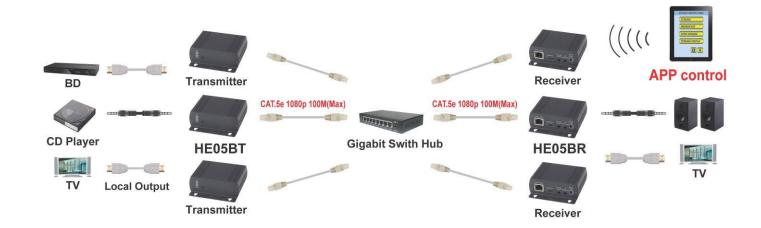
Recommend to use IGMP and Jumbo Frame over 8K Ethernet Switch Hub in order to achieve the best transmission quality
